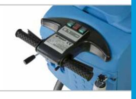
The shape of the instrument board, made of cast aluminium and injection moulded, facilitates machine control and guarantees the best visibility and safety of use
