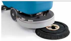
The washing unit of Minny 430-530-500 uses a single brush with a practical brush lock/unlock system requiring no manual intervention for installation.
