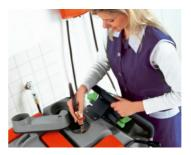
Automatic dosing- and filling system: Saves time when filling the tank, and the reduced consumption of cleaning detergents saves operating costs.
