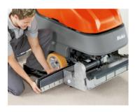
No pre-sweeping required, thanks to the integrated and easy-to-empty coarse dirt tray at the cylindrical brush unit (Scrubmaster B70 CL).
