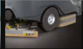
Rear/front super elastic wheels, for minimal vibration and increased comfort
